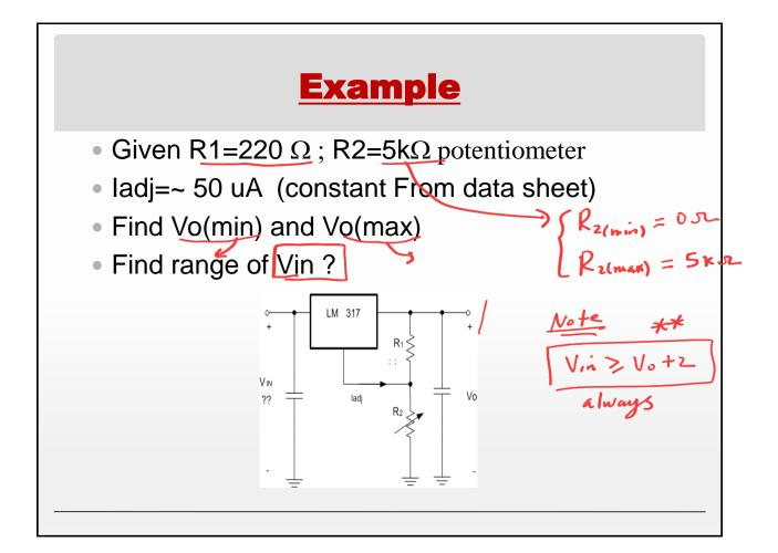
$$V_{0} = I_{REF} (R_{1}+R_{2}) + I_{n}d_{j}(R_{2})$$
